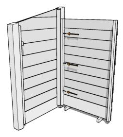
Begin by arranging the left panel (the one with the small wood block attached to the front post) and the back panel at 90° to each other, with the back panel raised up on the spacer blocks by approximately 25mm. Use 3 x shorter screws to secure as shown.
