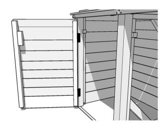
Returning to the front of the store, place the finishing strip against the 3 front posts as shown with the screw holes configured to create a triangle and slide it upwards until it is just touching the underside of the lid. Now fix in place with 3 x shorter green screws per post.
