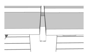
Lower the lid assemblies into place, the centre lid being the narrower one, and position them so that the hinge knuckles sit against the hinge strip... ..and there is a 15mm gap between the lid panels before fixing the hinges into place with 3 x black screws per hinge into the hinge strip.
