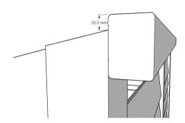
Stand the assembly back up and position the Hinge strip at the top of the rear posts...
