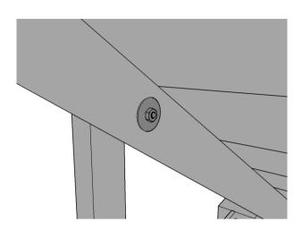
Take the coach bolt from the prop fixing and push it through the hole in the prop, add a washer and then push through the hole in the lid batten as shown.
