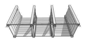
Carefully lay the assembly on its back and attach the metal bars, the centre bar being the shorter one, to the front bottom edge of the 3 front posts as shown, securing in place with 2 x shorter green screws per post.
