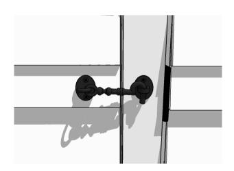
Position the cabin latch keep on the post and aligned horizontally with each latch as shown. Secure in place with 2 x black screws then repeat for the second and third door.
