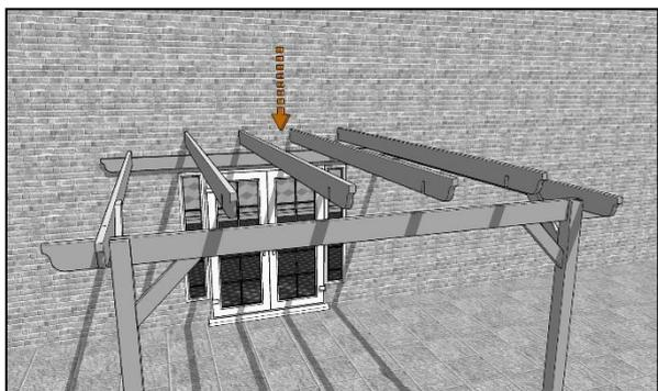
Using the marks on the runners as a guide, add the remaining rafters, securing each end in place with a 120mm coachscrew.
