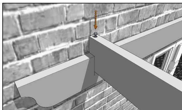
Make sure everything looks square and the rafter is aligned with the marks on the wall plate and fully slotted in place before securing into place with a 120mm coachscrew driven down through the rafter into the wall plate.
