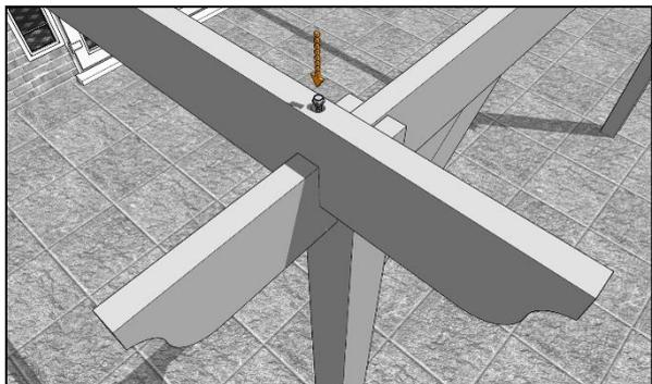
Then secure the other end to the runner using another 120mm coachscrew. Secure the other rafter in place before proceeding to step 10.
