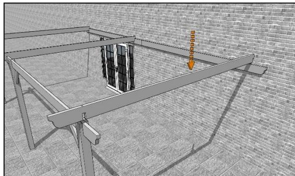
Now lower another rafter onto this end of the assembly, adjusting the post position if necessary, and once butted up to the outer face of the post and aligned on the wall plate marking, secure in place with a 120mm coachscrew at each end in the same way as you did for Steps 22 & 23.
