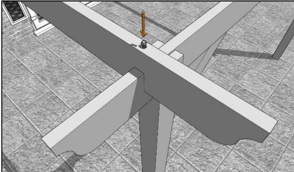
Then secure the other end to the runner using another 120mm coachscrew. Secure the other rafter in place before proceeding to step 24.
