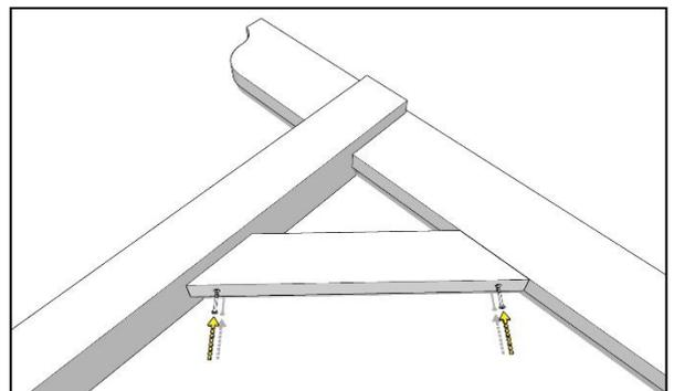
Add the short braces, butting their angled faces against the post and underside of the runner and aligning it centrally against the post before fixing into place with a 70mm woodscrew through each end. Attach both short braces in this way.
