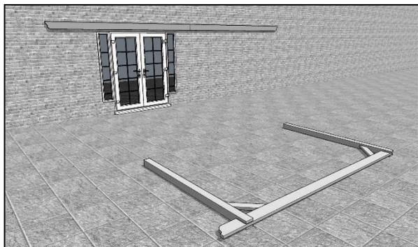
Get your assistants to manoeuvre the previously assembled "goalpost" assembly into place so that it is approximately in place, parallel to and about the length of a rafter away from the wall plate with the sculpted end outermost and opposite the sculpted end of the wall plate as shown...
