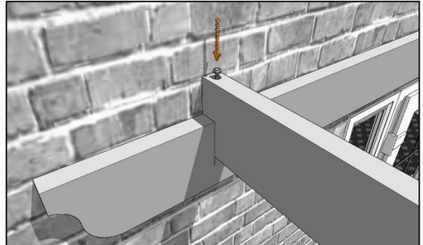
Make sure everything looks square and the outer rafter is aligned with the marks on the wall plate and fully slotted in place before securing into place with a 120mm coachscrew driven down through the rafter into the wall plate.
