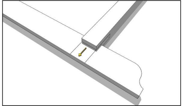
Lay one of the plain posts on a flat, level surface and then, using the marks on the runner as a guide, slot the runner on to it as shown.
