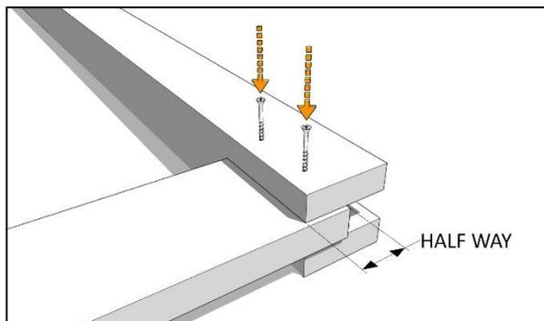
Take another post and slide it over the other (square) end of the runner so that it occupies half the width (around 47mm) of the slot in the post. Ensure it is square before securing in place with 2 of the 60mm screws
