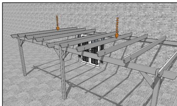
Finally, add the remaining rafters using the markings on the runners and wall plate as a guide, securing each one in place with a 120mm coachscrew down through each end, into the runner and wall plate.
