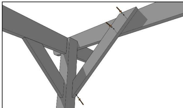
Now add the long braces, butting the angled face against the post and the bottom level with the short brace already installed. Fix the bottom end in place with a 70mm woodscrew and the top end in place with 2 of the 60mm woodscrews. Add the remaining 3 braces in the same manner.
