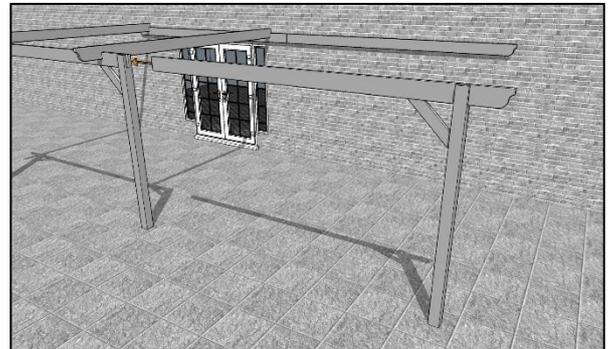
Take the completed frame assembly from Step 18 and slide the square rafter end into the central post slot as shown...
