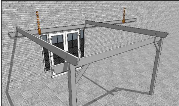
Lower the outer rafter so that it is slotted over the runner end wall plate/runner end, as close to the posts as possible and another slotted onto the runners at the marks closest to the central posts as shown above.
