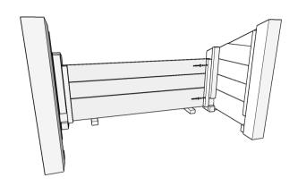
Begin by arranging the left panel and the back panel at 90° to each other, with the back panel raised up on the spacer blocks by approximately 25mm. Use 2 x Shorter green screws to secure as shown.
