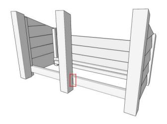
Now insert the back rail in the same manner, batten innermost, and secure each side in place with 2 x longer green screws.
