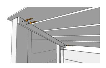
Lower the roof into place making sure that it is not back to front (check the roof battens finish flush with the outer posts).
