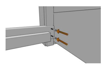
Now slide the front rail, vertical pencil marks outmost and the batten closest to the floor, into the slots toward the bottom of the front posts...
