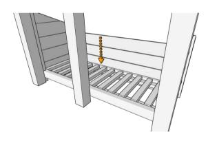
Fix the centre post in place with 2 x longer green screws driven through the front rail into the post.
