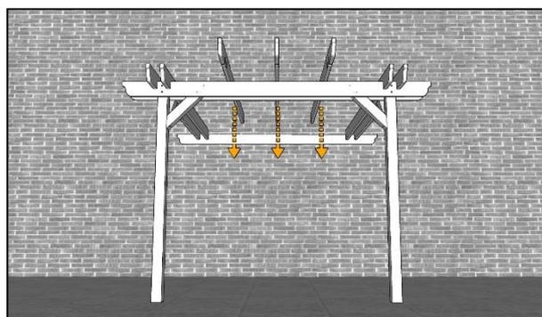
Drop the remaining rafters into place and secure in the same manner as before with a 120mm coachscrew at each end.
