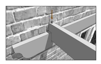
Make sure everything looks square and the outer rafter is aligned with the marks on the wall plate and fully slotted in place before securing into place with a 120mm coachscrew driven down through the rafter into the wall plate.
