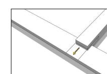
Work out where you wish to affix your wall plate, making sure that the area directly in front of it is flat, level and able to support the structure. Also check that the longer edge is at the top. Attach the wall plate using suitable fixings for the wall construction. Measure in 400mm from each end and use sufficient fixings so that the minimum distance between them is 500mm, distributed evenly and vertically centred across the wall. Ensure it is horizontal with a laser or spirit level.
