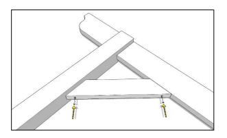
Add the short braces, butting their angled faces against the post and underside of the runner and aligning it centrally against the post before fixing into place with a 70mm woodscrew through each end. Attach both short braces in this way.
