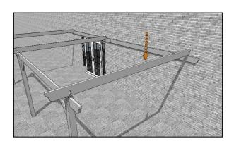
Now lower another rafter onto this end of the assembly, adjusting the post position if necessary, and once butted up to the outer face of the post and aligned on the wall plate marking, secure in place with a 120mm coachscrew at each end in the same way as you did for Steps 22 & 23.
