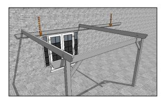
Lower the outer rafter so that it is slotted over the runner end wall plate/runner end, as close to the posts as possible and another slotted onto the runners at the marks closest to the central posts as shown above.
