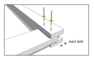
Take another post and slide it over the other (square) end of the runner so that it occupies half the width (around 47mm) of the slot in the post. Ensure it is square before securing in place with 2 of the 60mm screws
