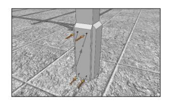
If you are fitting cladding panels, line up each panel as shown, ensuring that it is vertical and the edges align with the post before secure each panel in place with a 60mm wood screw in each corner. Attach to each face of the post or as necessary.
