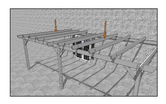
Finally, add the remaining rafters using the markings on the runners and wall plate as a guide, securing each one in place with a 120mm coachscrew down through each end, into the runner and wall plate.
