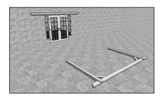
Get your assistants to manoeuvre the previously assembled "goalpost" assembly into place so that is it approximately in place, parallel to and about the length of a rafter away from the wall plate...
