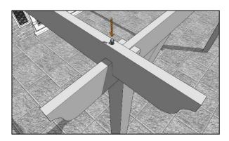
Then secure the other end to the runner using another 120mm coachscrew. Secure the other rafter in place before proceeding to step 10.
