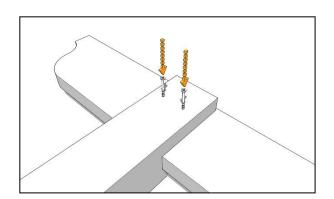
Make sure the post is correctly aligned and square to the runner before securing into place with 2 of the 60mm woodscrews. Repeat this process for the other end of the runner.
