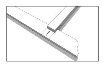
Lay one of the plain posts on a flat, level surface and then, using the marks on the runner as a guide, slot the runner on to it as shown.
