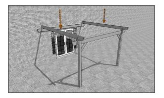
Drop the 2 outer rafters into place, making sure they are butted up against the outer end face of the posts.
