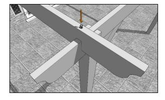
Then secure the other end to the runner using another 120mm coachscrew. Secure the other rafter in place before proceeding to step 24.
