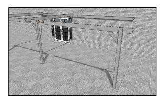
Take the completed frame assembly from Step 18 and slide the square rafter end into the central post slot as shown...
