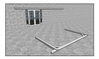
Get your assistants to manoeuvre the previously assembled "goalpost" assembly into place so that is it approximately in place, parallel to and about the length of a rafter away from the wall plate with the sculpted end outermost and opposite the sculpted end of the wall plate as shown...
