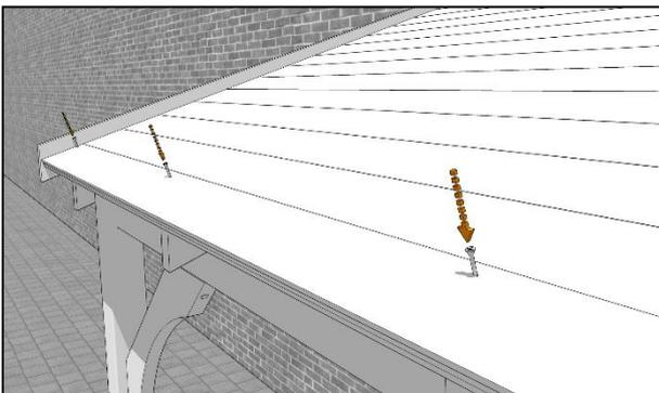
Add the final tongue and groove panel before fixing into place with a 60mm into each rafter spaced 20mm from the top edge of the panel.
