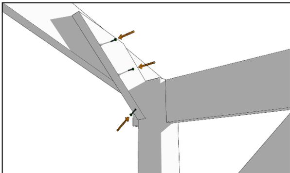
Place an end brace against the inner face of the outer runner so that the lower face is butted against the inner face of the post and the top edge is approximately 10mm from the top edge of the rafter. Fix in place with 2 x 50mm coachscrews into the rafter and 1 x 70mm screw into the post as shown. Repeat for the other end of the structure.
