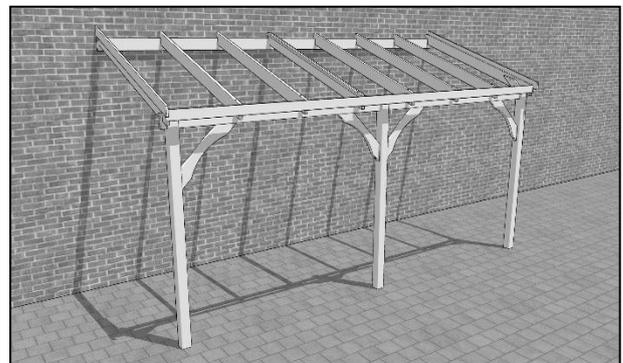
Now add the remaining plain rafters, using the markings on the runner and wall plate and fixing into place with a 120mm coachscrew into the wall plate and runner as before.
