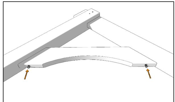
Align a brace with the underside of either end of the runner and centrally across the inside face of the post as shown. The mating faces should be flat against each other before fixing the brace into place with a 70mm coachscrew at each end. Repeat and attach the remaining brace to the other end of the runner to form a "goal post" structure.
