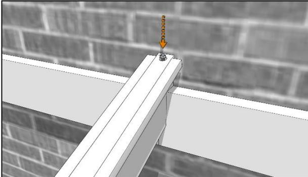
Now fix the intermediate rafter (it has battens attached to either side) into place with a 120mm coachscrew driven down into the centre of the wall plate...
