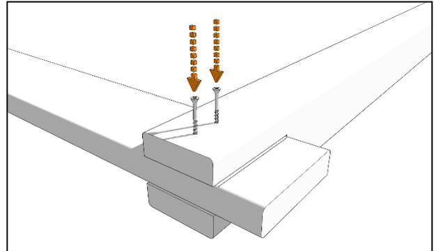
Place one of the single slotted posts on a flat surface as shown and then insert one of the runners into the post slot, using the markings on the runner as a guide. Fix into place with 2 x 60mm woodscrews.
