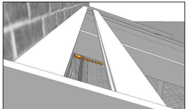
Slide a tongue and groove panel up the rafters and fully locate the tongue into the ridge piece...
