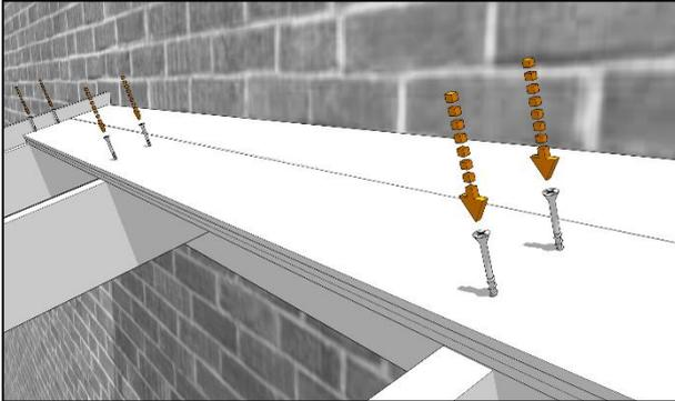
...before fixing into place with 2 x 60mm screws into each rafter, spaced 20mm from the upper and lower edges.
