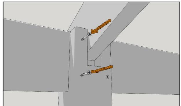
... before securing it into place with 2 x 60mm screws through the post into the runner.
