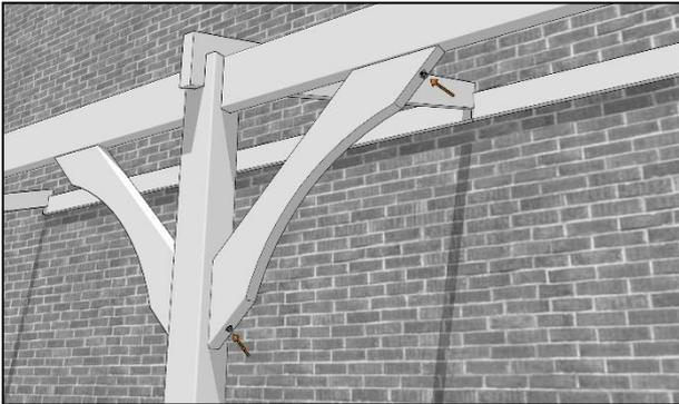
Now fit the final brace into place, Aligning it the underside of the runner and centrally across the inside face of the post. Fix it into place with a 70mm coachscrew at each end.
