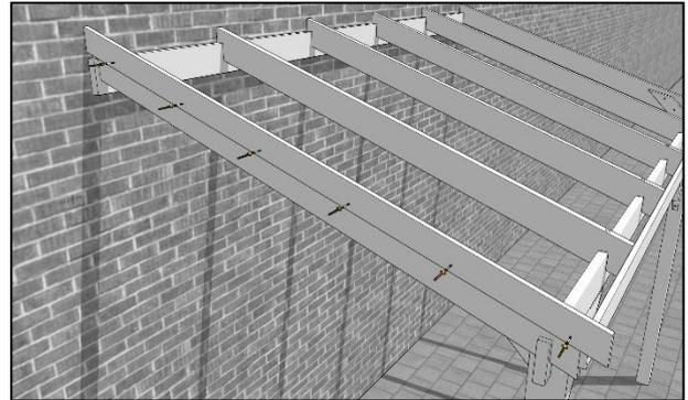
...and fix into place with 50mm screws evenly spaced around 600mm apart.
