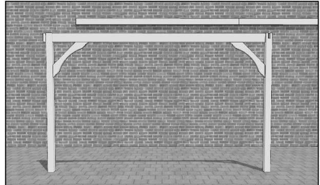
Using your assistants, manoeuvre the previously assembled “goalpost” with 2 posts into place. Position it parallel to the wall with the central post adjacent to the centre of your wall plate(s). Consult the Roof depth reference table (page 3) to correctly distance the posts from the wall.
