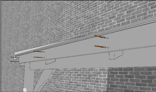
Slot a fascia panel into place so that it is butted up against the underside of the roof and against the rafter ends before fixing in place with 2 x 60mm screws into the rafter ends. Repeat for the second fascia panel and then proceed to the Shingle installation after affixing the cladding panels.
