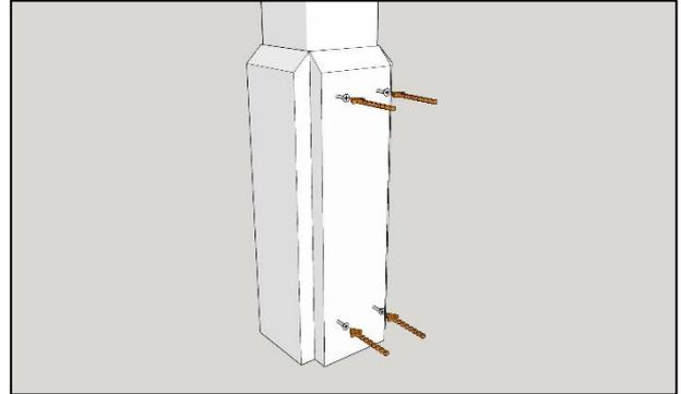
To attach cladding panels simply align as shown at the base of the post before screwing into place using 4 x 60mm woodscrews through the pre-drilled holes per panel. Repeat for each face of the post.
