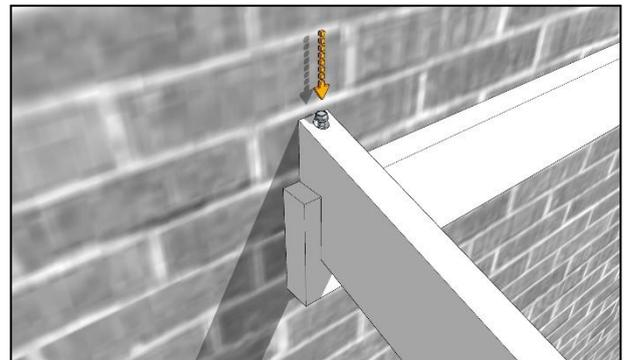
Adjust the positioning of the “goal post” if necessary, so that the notch in the underside of the wall end of the outer rafter sits snugly on the top of the wall plate and also lines up with the markings indicating its correct position. Fix in place with a 120mm coachscrew driven down into the wall plate.
