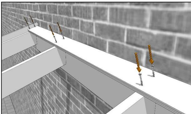
Take the tongue and groove ridge (with no tongue), groove side facing down the roof and position it at the top of the rafters before fixing into place with:
