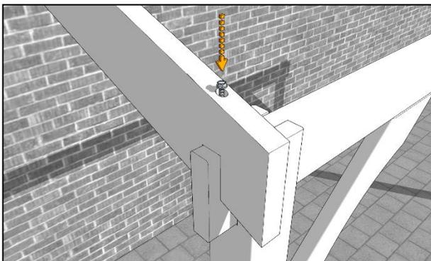
Butt the outer rafter against the outer face of the post before securing in place with a 120mm coachscrew driven down into the runner.
