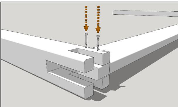
Slot a double slotted post over the other end of the runner, aligning with the single mark on the runner top edge and fix into place with 2 x 60mm woodscrews.
