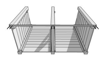
Carefully lay the assembly on its back and attach the metal bars to the front bottom edge of the 3 front posts as shown, securing in place with 2 x shorter green screws per post.
