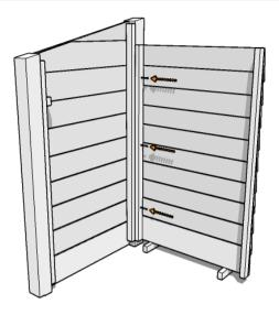
Begin by arranging the left panel (the one with the small wood block attached to the front post) and the back panel at  $90^\circ$  to each other, with the back panel raised up on the spacer blocks by approximately 25mm. Use 3 x shorter green screws to secure as shown.
