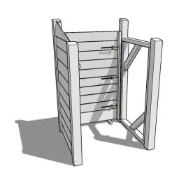
Now add the Dividing frame, fixing in the same way with 3 x shorter green screws.
