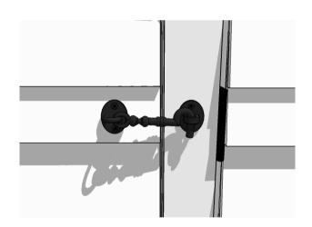
Position the cabin latch keep on the post and aligned horizontally with the latch as shown. Secure in place with 2 x black screws then repeat for the second door.
