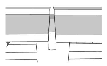
Lower the lid assemblies into place and position them so that the hinge knuckles sit against the hinge strip...
