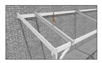
Now add the intermediate rafters, using the markings on the runner and wall plate...
