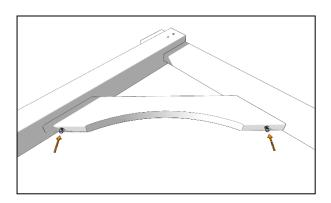
Align a brace with the underside of either runner and centrally across the inside face of the post as shown. The mating faces should be flat against each other before fixing the brace into place with a 100mm coachscrew at each end. Repeat and attach the remaining brace to the other end of the runner to form a "goal post" structure.
