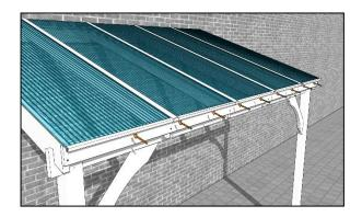
Slot a panel closure strip onto the end of each panel and a glazing bar cap onto the end of each cap.
