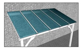
Continue adding further panels as you did in Step 21 and finish off with the other drilled panel, fixed in place with roofing screws as you did with the first panel in Step 18.
