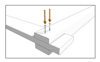
Place one of the single slot posts on a flat surface as shown and then insert one of the runners into the post slot, using the markings on the runner as a guide. Fix into place with 2 x 75mm woodscrews.
