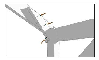
Place an end brace against the inner face of the outer runner so that the lower face is butted against the inner face of the post and the top edge is approximately 10mm from the top edge of the rafter. Fix in place with 2 x 50mm coachscrews into the rafter and 1 x 100mm coachscrew into the post as shown.
