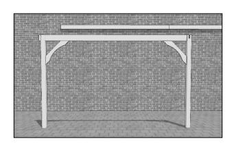
Using your assistants, manoeuvre the previously assembled "goalpost" with 2 posts into place. Position it parallel to the wall with the 4 slot post adjacent to the centre of your wall plates. Consult the Panel length table (page 4) to correctly distance the posts from the wall.
