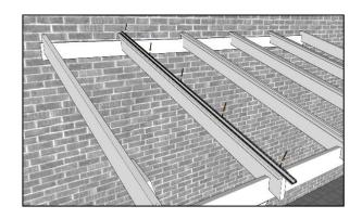
Starting from one end of the car port attach the previously drilled glazing bar so that it is centred on the first inner rafter and butted up to the wall as shown. Fix in place with 60mm screws.
