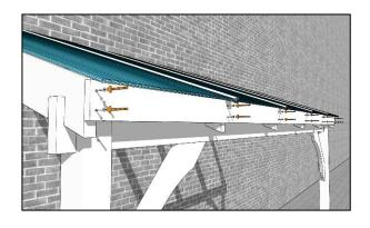
Position the fascia so that its ends are flush with outer rafters and its top edge is just touching the underside of the glazing bars. Fix into place with a pair of 60mm screws into the rafter ends.
