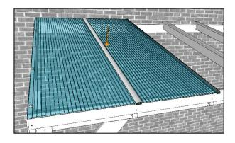
Add the next glazing bar as before, centred on the rafter and butted against the wall. Add an undrilled panel, aluminium tape at the wall and UV coated side up, adjacent to the last panel and use an assistant to support the lower panel edge whilst the glazing bar capping is snapped into place on the first glazing bar as shown.
