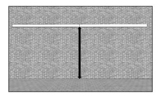
Begin by taking the wall plates, one at a time, and placing them horizontally (use a spirit level or laser) on the wall where you would like the car port located. Check the Panel length table (page 4) to establish the distance from TOP of the wall plates to the floor. Mark the hole positions for your wall fixings then drill and fix them into place.
