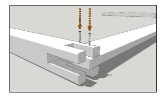
Slot the centre post with the double slot over the other end of the runner, aligning with the single mark on the runner top edge and fix into place with 2 x 60mm woodscrews.
