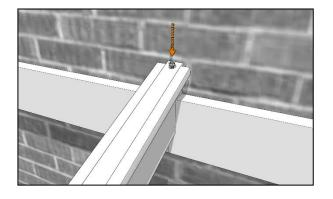
...before fixing each end into place with a 120mm coachscrew.
