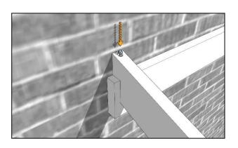
Adjust the positioning of the "goal post" if necessary, so that the notch in the underside of the wall end of the outer rafter sits snugly on the top of the wall plate and also lines up with the markings indicating its correct position. Fix in place with a 120mm coachscrew driven down into the runner.
