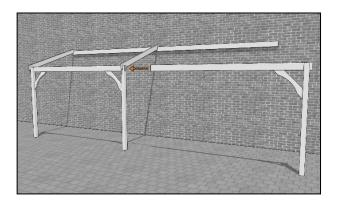
Using your assistants again, manoeuvre the previously assembled "goal post" with 1 post into place. Slide the free runner end into the slot in the centre post pushing it fully home until it butts against the other runner...
