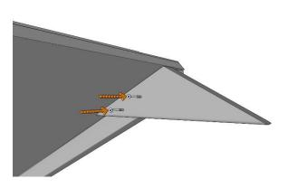
Take one of the roof panels and line up a roof gusset as shown with the apex adjacent to the edge of the roof panel and butted up against the inner edge of the roof batten...
