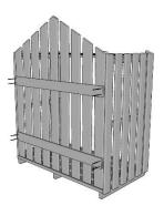
Now lower the shelf into place, gently easing the side panels apart, if necessary, until it is located on its supports as shown.
