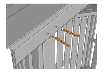
...ensuring the roof battens fit over the front and back as shown here.
