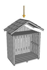
Add the second roof panel, butting it up to the first one and fix into place with another 2 x 40mm screws through each of the gussets as shown for each side.
