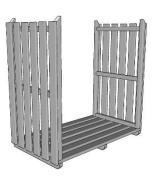
...and fix into place with 3 x 100mm screws as shown.
