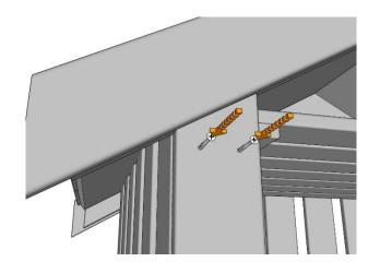
Line up an eave panel so that centremost end is aligned with the roof panel joint and the face is vertical. Fix into place with 3 x 40mm screws as shown. Repeat for the other side, making sure to butt the centre join together. Now repeat the process on the rear of the store.
