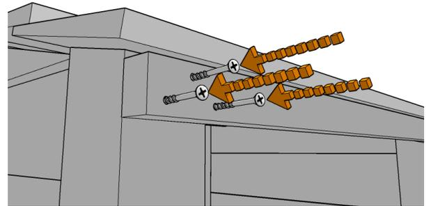
...until it is just touching the underside of the lid. Now fix both ends in place with 3 x 65mm screws per post.
