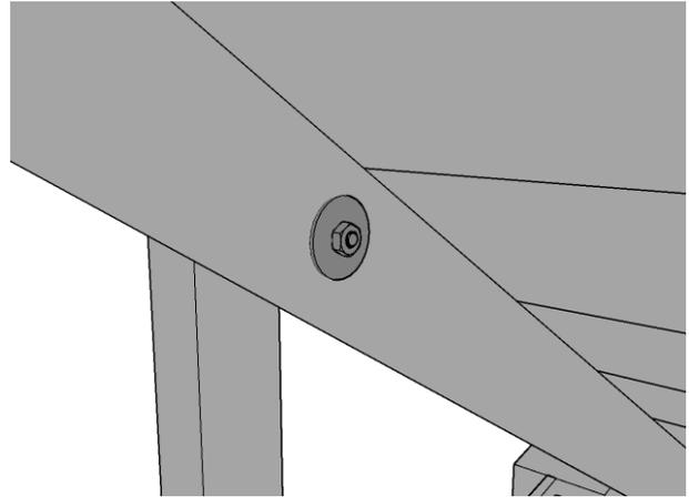
Place another washer over the coach bolt and finally the securing nut. Tighten with a spanner or socket until fully tight and then back off until the prop is able to swing freely.
