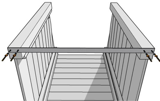
Carefully lay the assembly on its back and attach the metal bar to the front bottom edge of the 2 front posts as shown, securing in place with 2 x 65mm screws per post.
