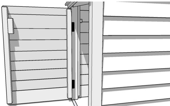
Align the door (hinge side on the left) so that the top edge clears the underside of the finishing strip by approx 10mm and each hinge leaf sits flat against the post with the knuckles resting against the front edge of the post. Secure the hinges in place using 8 x black screws.
