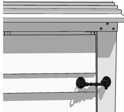
Position the cabin latch keep on the post and aligned horizontally with the latch as shown. Secure in place with 2 x black screws.
