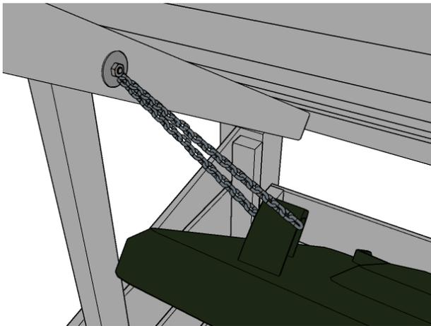
If your bin lid has a suitable handle you may use the chain provided to attached this to the store lid. Undo the nut and slip one end over the coachbolt, then pass other end through the handle and then over the end of the coach bolt, pulling chain through until it is tight enough. Now re-attach the nut.
