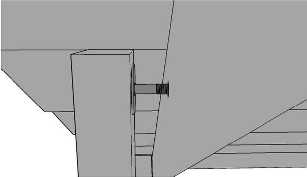
Take the coach bolt from the prop fixing and push it through the hole in the prop, add a washer and then push through the hole in the lid batten as shown.
