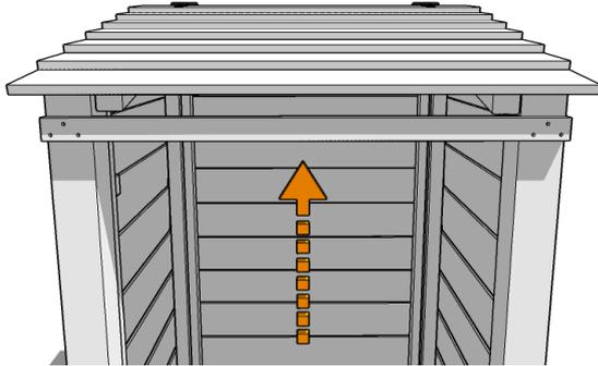
Returning to the front of the store, place the finishing strip against the 2 front posts as shown with the screw holes configured to create a triangle and slide it upwards...
