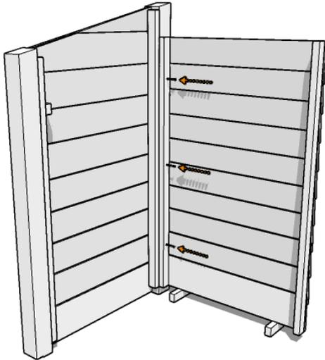
Begin by arranging the left panel (the one with the small wood block attached to the front post) and the back panel at 90° to each other, with the back panel raised up on the spacer blocks by approximately 25mm. Use 3 x 65mm screws to secure as shown.
