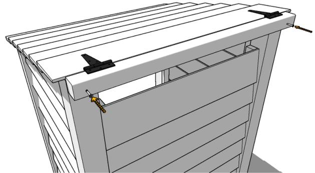
Stand the assembly back up and lower the lid assembly into place so that the hinge bar is centred across the rear posts and fix into place with a 75mm screw into each post.
