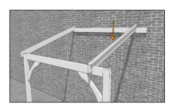
Add the intermediate rafter, using the markings closest to the centre post on the runner and wall plate, adjusting the position of the "goal post" as necessary. Do not fix in place at this stage.
