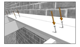
...before fixing into place with 2 x 45mm screws into each rafter, spaced 20mm from the upper and lower edges.
