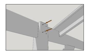
$\dots$  before securing it into place with 2 x 65mm screws through the post into the runner.
