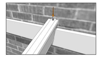
Now fix the intermediate rafter into place with a 120mm coachscrew driven down into the wall plate...
