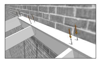
Take the short tongue and groove ridge (with no tongue), groove side facing down the roof and position it at the top of the rafters before fixing into place with:
