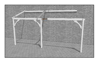
Using your assistants again, manoeuvre the previously assembled "goal post" with 1 post into place. Slide the free runner end into the slot in the centre post pushing it fully home until it butts against the other runner...
