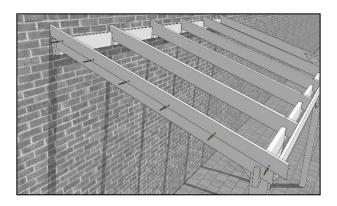
...and fix into place with 45mm screws.
