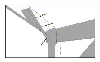
Place an end brace against the inner face of the outer runner so that the lower face is butted against the inner face of the post and the top edge is approximately 10mm from the top edge of the rafter. Fix in place with 2 x 65mm screws into the rafter and 1 x 75mm screw into the post as shown. Repeat for the other end of the structure.
