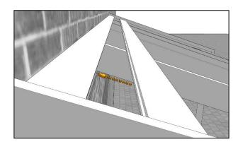
Slide a short tongue and groove panel up the rafters and fully locate the tongue into the ridge piece...
