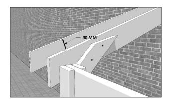
Position the end cover so that its rear edge is butted against the wall and the top edge is 30mm above the roof panel...
