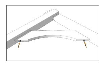
Align a brace with the underside of either end of the runner and centrally across the inside face of the post as shown. The mating faces should be flat against each other before fixing the brace into place with a 100mm coachscrew at each end. Repeat and attach the remaining brace to the other end of the runner to form a "goal post" structure.
