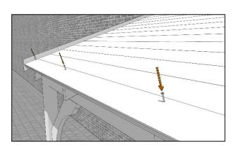
Add the final short tongue and groove panel before fixing into place with a 45mm into each rafter spaced 20mm from the top edge of the panel.
