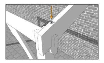
Drop the remaining outer rafter into place and fix into place as you did in steps 9 & 10.
