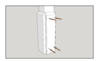
To attach cladding panels simply align as shown at the base of the post before screwing into place using 4  $\times$  65mm woodscrews through the pre-drilled holes per panel. Repeat for each face of the post.
