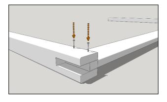
Slot another post over the other end of the runner, aligning with the single mark on the runner top edge and fix into place with 2 x 60mm woodscrews.
