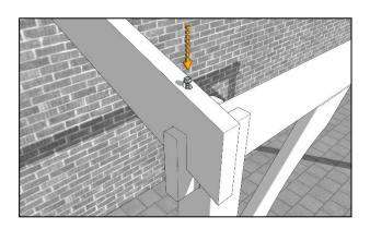
Butt the other rafter against the outer face of the post before securing in place with a 120mm coachscrew driven down into the runner.
