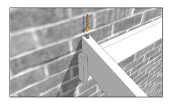
Adjust the positioning of the "goal post" if necessary, so that the notch in the underside of the wall end of the outer rafter sits snugly on the top of the wall plate and also lines up with the markings indicating its correct position. Fix in place with a 120mm coachscrew driven down into the wall plate.
