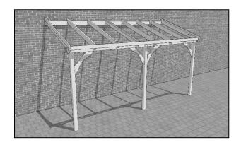
Now add the remaining rafters, using the markings on the runner and wall plate and fixing into place with a 120mm coachscrew into the wall plate and runner as before.
