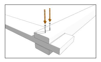
Place one of the posts on a flat surface as shown and then insert one of the runners into the post slot, using the markings on the runner as a guide. Fix into place with 2 x 75mm woodscrews.
