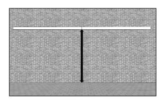
Begin by taking the wall plate(s) and placing it/them horizontally (use a spirit level or laser) on the wall where you would like the car port located. Check the Panel length table (page 4) to establish the distance from TOP of the wall plates to the floor. Mark the hole positions for your wall fixings then drill and fix them into place.
