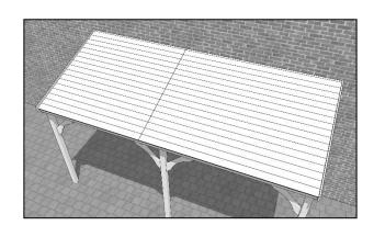
Slot the fascia panel into place so that it is butted up against the underside of the roof and against the rafter ends before fixing in place into the outer rafter at both ends with  $2 \times 45 \text{mm}$  screws ...
