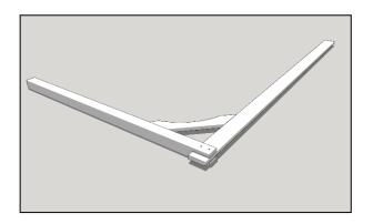
Assemble the second "goal post" using the remaining post, runner and brace in the same manner as before.
