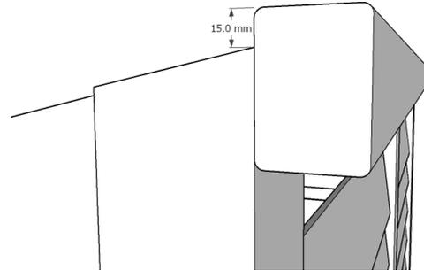
...set the hinge bar so that the top edge sits approx. 15mm above the top of the rear post and secure in place with a 75mm screw into each of the 3 posts.
