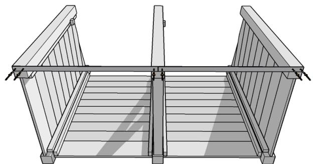
Carefully lay the assembly on its back and attach the metal bars to the front bottom edge of the 3 front posts as shown, securing in place with 2 x 65mm screws per post.
