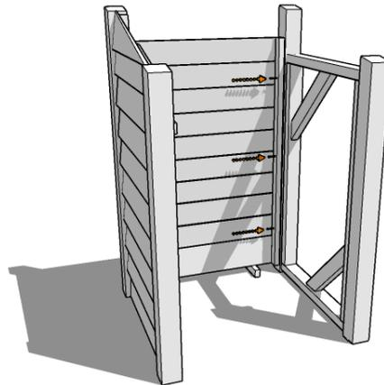
Now add the Dividing frame, fixing in the same way with 3 x 65mm screws.
