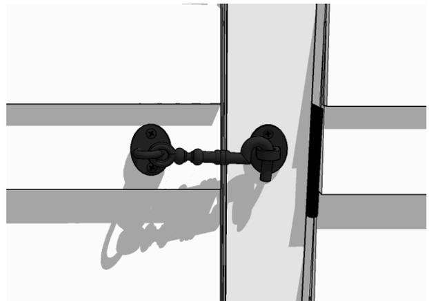
Position the cabin latch keep on the post and aligned horizontally with the latch as shown. Secure in place with 2 x black screws then repeat for the second door.
