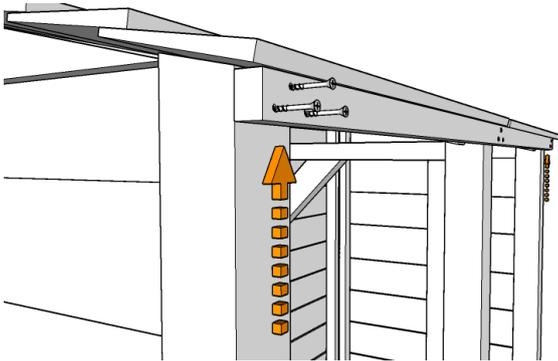
Returning to the front of the store, place the finishing strip against the 3 front posts as shown with the screw holes configured to create a triangle and slide it upwards until it is just touching the underside of the lid. Now fix in place with 3 x 65mm screws per post.
