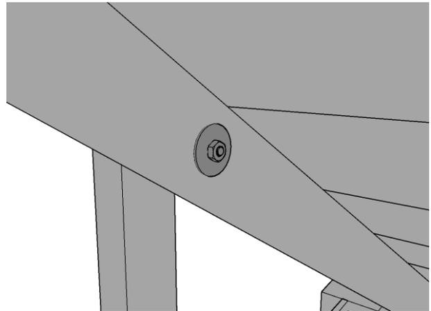
Place another washer over the coach bolt and finally the securing nut. Tighten with a spanner or socket until fully tight and then back off until the prop is able to swing freely. Attach the second prop in the same manner.
