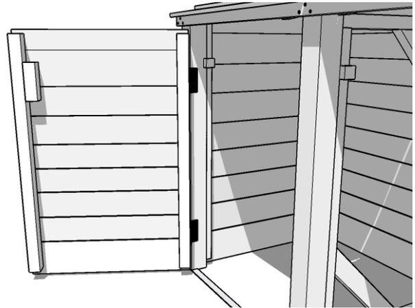
Align the door (hinge side on the left) so that the top edge clears the underside of the finishing strip by approx 10mm and each hinge leaf sits flat against the post with the knuckles resting against the front edge of the post. Secure the hinges in place using 8 x black screws.
