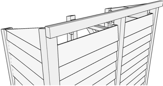
Stand the assembly back up and position the Hinge strip at the top of the rear posts...
