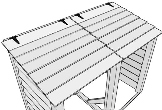
Lower the lid assemblies into place and position them so that the hinge knuckles sit against the hinge strip...
