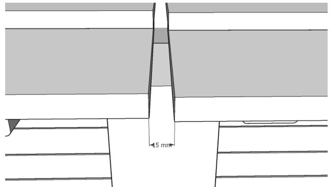
..and there is a 15mm gap between the lid panels before fixing the hinges into place with 3 x black screws per hinge into the hinge strip.
