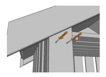
Line up an eave panel so that centremost end is aligned with the roof panel joint and the face is vertical. Fix into place with 3 x 40mm screws as shown. Repeat for the other side, making sure to butt the centre join together. Now repeat the process on the rear of the store.
