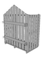
Now lower the shelf into place, gently easing the side panels apart, if necessary, until it is located on its supports as shown.
