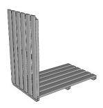
Begin by placing the base in position close to the intended final location with the chamfered supports ends facing front as shown.
