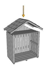
Add the second roof panel, butting it up to the first one and fix into place with another 2 x 50mm screws through each of the gussets as shown for each side.
