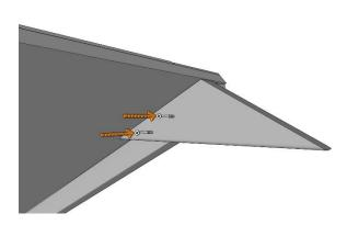
Take one of the roof panels and line up a roof gusset as shown with the apex adjacent to the edge of the roof panel and butted up against the inner edge of the roof batten...
