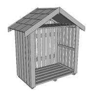
Place the flashing strip onto the apex of the roof and secure with the 4 x dome head screws as shown.
