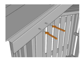
Fix the roof into place into the at each corner with 2  $\times$  60mm screws.
