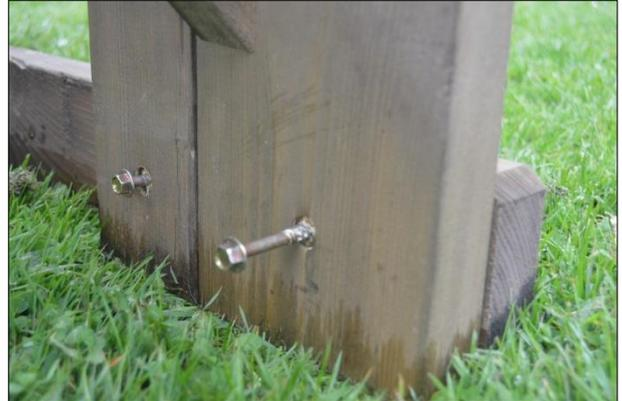
... and fix into place using 2 x 60mm coach screws. Repeat this for the remaining 3 seat frame ends.
