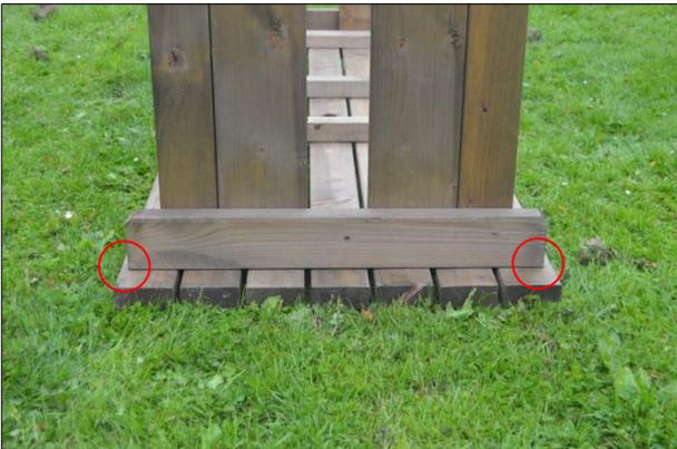
Place one of the table leg frames centrally against the fixing batten ensuring that the gap at the table edge is the same on both sides. Now, using 2 of the supplied 70mm coach screws and the pre drilled holes, secure the table leg frame to the fixing batten on the table top.
