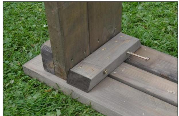
Attach the leg frame using 2 x 70mm coach screws as shown. Repeat for the other end of the seat panel then for the remaining seat panel and leg frames. (For the junior/children's version proceed to Step 28)
