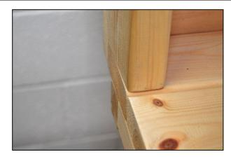
To attach a back rest place it, resting on the rear of the work bench as shown, with each end flush with the table top ends...
