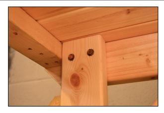
...and working from underneath the top ensure the top of each leg is located as shown, butted against the inner edges of the top before fixing each leg into place with 2 x 60mm coach screws.
