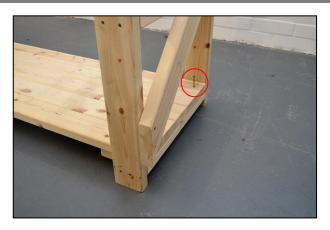
Ensure the end of the shelf is flush with the leg assembly and secure into place at the front and rear of the shelf with a 65mm screw at each corner. (45mm screw for MDF version)
