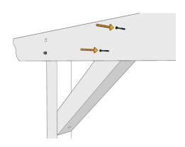
Once the brace is in position insert 2  $\times$  70mm coachscrews and fix it to the post by driving them fully home with the socket.
