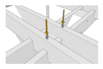
Now insert the remaining pre-drilled rafters adjacent to the rafters inserted previously.
