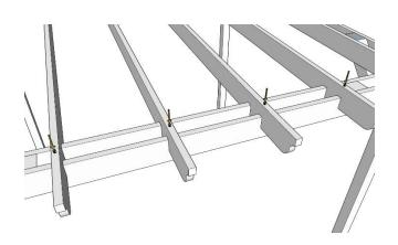
Now insert any remaining rafters using the lines marked on the top face of the runner to space them correctly...
