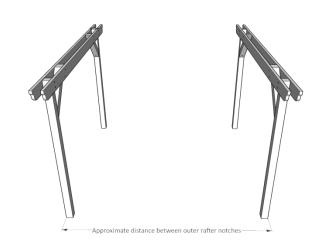
Place the next runner as you did before carefully aligning it before attaching to the post and brace as before.
