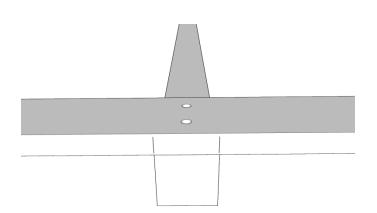
Begin by placing two of the posts on a flat surface as shown and then placing one of the runners, countersinks uppermost, on top of the posts.
