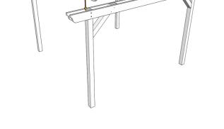
Now take one of the pre-drilled rafters and lower it onto the 2 frame assemblies so that the notches in the rafters and runners interlock and fully house. **Tip:** You may need to adjust the positioning of the frames in relation to each other to get everything square and true for this and the following stage. Drop a second pre-drilled rafter into place at the other end of the assembly.
