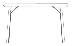
Insert a second 70mm coachscrew into the hole in the runner and drive both coachscrews fully home. Repeat the previous steps and attach the second post to the runner.
