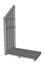
Begin by placing the base in position close to the intended final location with the chamfered supports ends facing front as shown.
