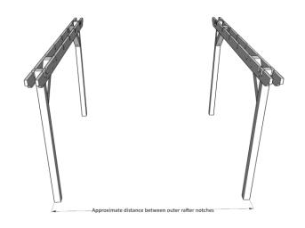
Place the next runner as you did before carefully aligning it before attaching to the post and brace as before.
