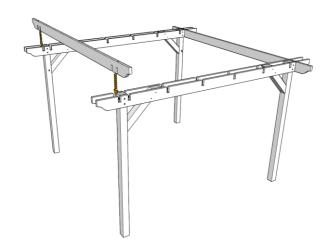
Now take one of the pre-drilled rafters and lower it onto the 2 frame assemblies so that he notches in the rafters and runners interlock and fully house.
