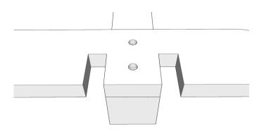
Begin by placing two of the posts on a flat surface as shown and then placing one of the runners, countersinks uppermost, on top of the posts with the outer notches over the post. At this point ensure that the post is aligned between the notches, flush with the top edge of the runner and perpendicular to it.
