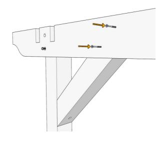
Once the brace is in position insert 2 x 70mm coachscrews and fix to the post by driving them fully home with the socket.
