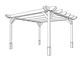
To attach cladding panels simply align as shown at the base of the post before screwing into place using 4 x 65mm woodscrews through the pre-drilled holes per panel. Repeat for each face of the post.
