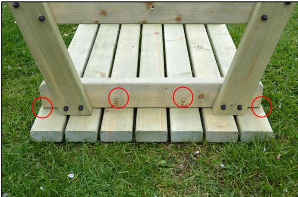
Place one of the table A-frames centrally against the fixing batten ensuring that the gap at the table edge is the same on both sides. Now, using 2 of the supplied 70mm coach screws and the pre drilled holes, secure the table A-frame to the fixing batten on the table top.
