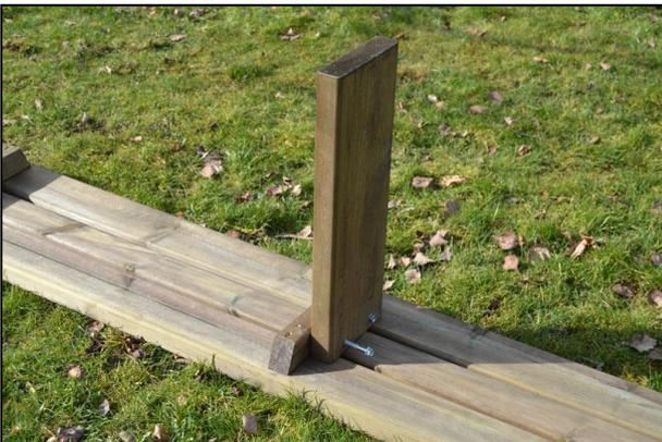
For a 7 or 8ft model, follow Steps 7 to 10. Place one of the seat panels upside on a flat surface and place the seat support adjacent to the centre batten...
