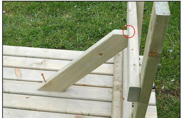
Place a cross brace in position as shown, ensuring that it is flush with the underside of the table A-frame and proceed to step 5.
