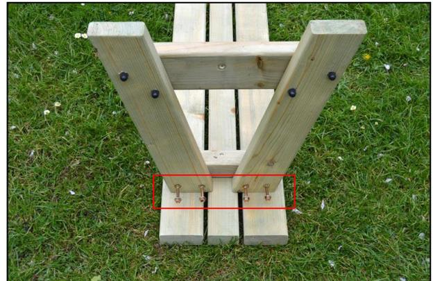
Place one of the bench A-frames centrally against the fixing batten ensuring that the gap at the bench edge is the same on both sides. Now, using 4 of the supplied 60mm coach screws and the pre drilled holes, secure the bench A-frame to the fixing batten on the seat and repeat for the remaining 3 A- frames.
