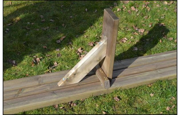
...before fixing into place with a 60mm coach screw through the brace into both the seat support and the underside of the seat panel. Add a second brace to the other side of the support in the same way. Repeat steps 9 to 12 for the remaining seat.
