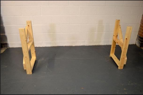
Start by placing the 2 leg assemblies, spaced approximately the length of your bench apart, facing each other, ensuring that they are correctly oriented as shown with the braces outermost and their lower end towards the front.
