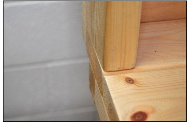
To attach a back rest place it, resting on the rear of the work bench as shown, with each end flush with the table top ends...
