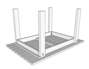
Place an M8 washer and nut onto each bolt and fully tighten.
