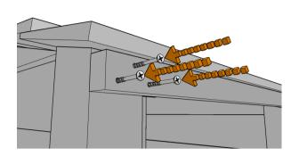
Returning to the front of the store, place the finishing strip against the 2 front posts as shown with the screw holes configured to create a triangle and slide it upwards...
