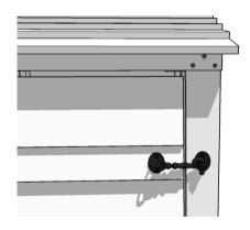
Align the door (hinge side on the left) so that the top edge clears the underside of the finishing strip by approx 10mm and each hinge leaf sits flat against the post with the knuckles resting against the front edge of the post. Secure the hinges in place using 8 x black screws.
