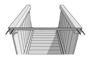
Carefully lay the assembly on its back and attach the metal bar to the front bottom edge of the 2 front posts as shown, securing in place with 2 x shorter green screws per post.
