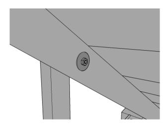
Take the coach bolt from the prop fixing and push it through the hole in the prop, add a washer and then push through the hole in the lid batten as shown.
