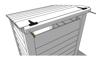
Stand the assembly back up and lower the lid assembly into place so that the hinge bar is centred across the rear posts and fix into place with a longer green screw into each post.
