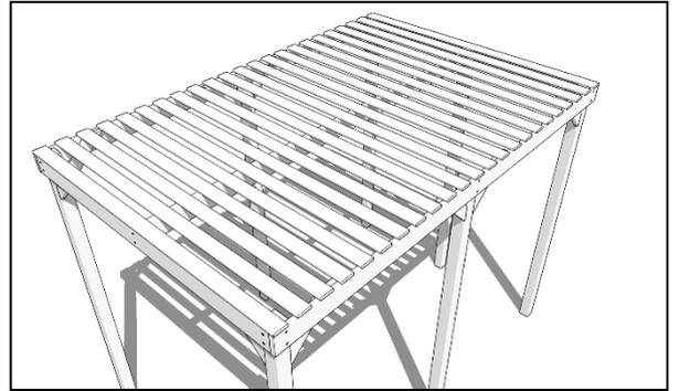
Continue adding the rest of the roof slats in the same manner until it is complete – as you approach the final 4-5 slats, manually equalise the spacing to allow for machining tolerances of the timber.
