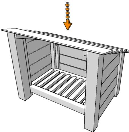
Lower the roof into place making sure that it is not back to front (check the roof battens finish flush with the outer posts).
