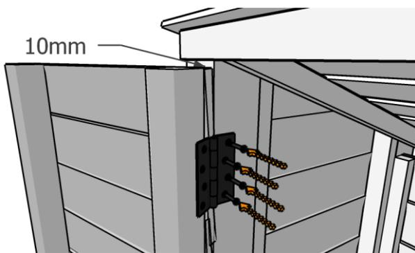
Align each door (also check it is the right way up) so that the top edge clears the underside of the finishing strip by approx 10mm and each hinge leaf sits flat against the post with the knuckles resting against the front edge of the post. Secure the hinges in place using 8 x black screws.
