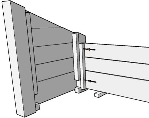
Begin by arranging the left panel and the back panel at 90° to each other, with the back panel raised up on the spacer blocks by approximately 25mm. Use 2 x shorter green screws to secure as shown.
