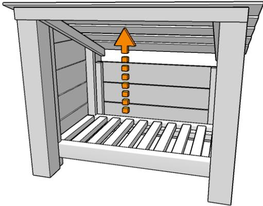
Place the finishing strip flat against the front posts so that it is centred across them. Now slide it up until it just touches the underside of the roof.
