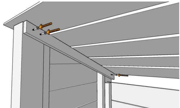
Now fix both sides of the roof into place with 2 x shorter green screws into the front post and 1 x shorter green screw into the rear post.
