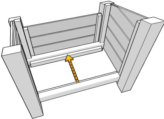
Now insert the other rail in the same manner, batten innermost, and secure each side in place with 2 x longer green screws.
