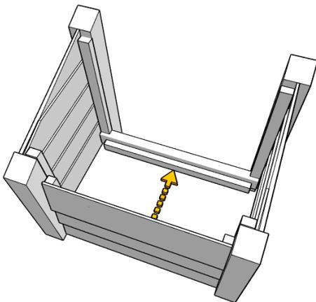
Now slide a rail, batten closest to the floor and innermost, into the slots toward the bottom of the front posts...
