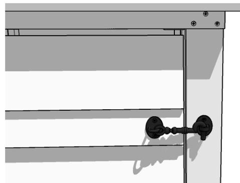
Position a cabin latch keep on the post and aligned horizontally with the latch as shown. Secure in place with 2 x black screws.
