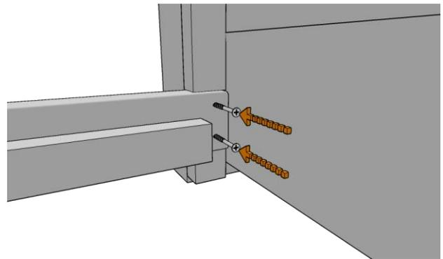
...and secure each side in place with 2 x longer green screws per side.
