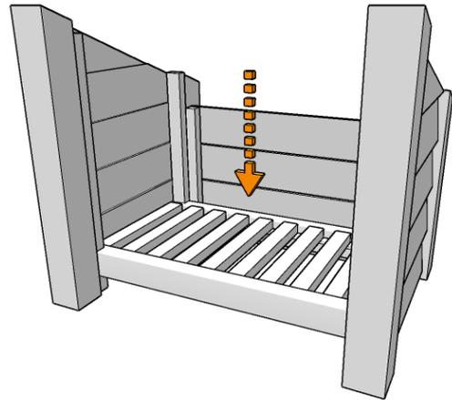
Drop the lattice into place so that it is sitting on the batters of the rails.
