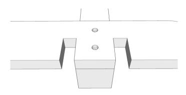
Begin by placing two of the posts on a flat surface as shown and then placing one of the runners, countersinks uppermost, on top of the posts with the outer notches over the post.
