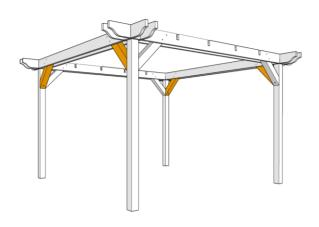
Now insert the remaining pre-drilled rafters adjacent to the rafters inserted previously.
