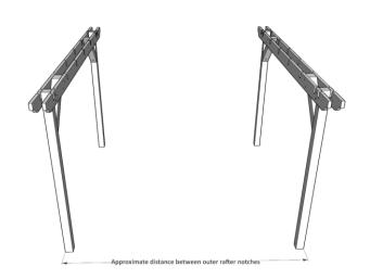
Repeat steps 1 - 9 so that you now have two frame assemblies. Arrange them both near to the pergola's intended final location, as shown above, spacing the posts apart by the approximate distance between the outer rafter notches.
