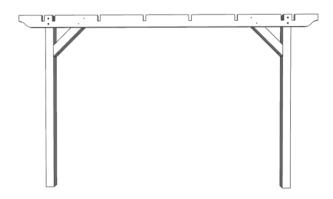
Insert a second 70mm coachscrew into the hole in the runner and drive both coachscrews fully home. Repeat the previous steps and attach the second post to the runner.
