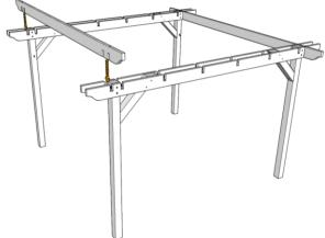
Drop a second pre-drilled rafter into place at the other end of the assembly.
