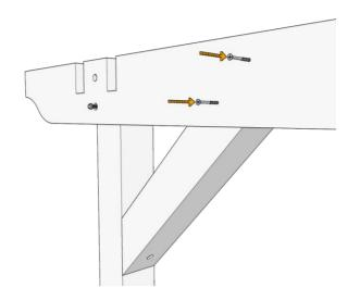
Once the brace is in position insert 2 x 70mm coachscrews and fix to the post by driving them fully home with the socket.
