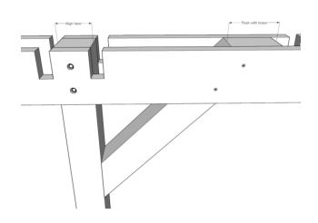
Place the next runner as you did before carefully aligning it before attaching to the post and brace as before.
