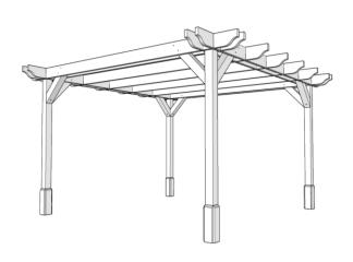
To attach cladding panels simply align as shown at the base of the post before screwing into place using  $4 \, x$  green woodscrews through the pre-drilled holes per panel. Repeat for each face of the post.
